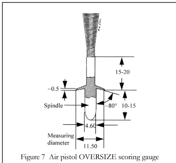
Figure 7 Air pistol OVERSIZE scoring gauge
