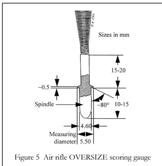
Figure 5 Air rifle OVERSIZE scoring gauge
